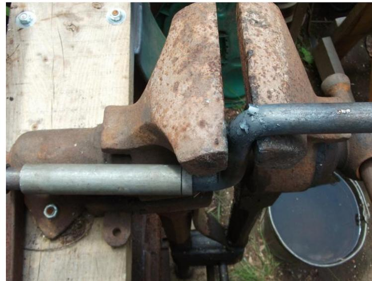
Heat and bend – remember to slide on the stops and the rolling sleeve first. The bucket of water is to cool the last bend each time.
