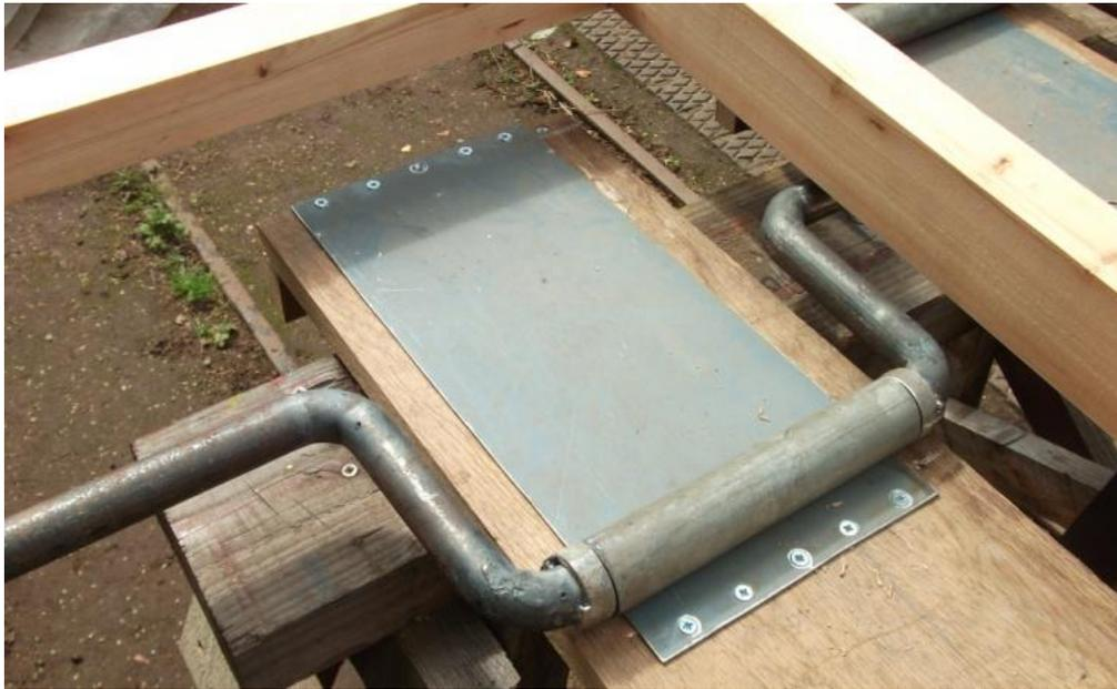
The backs of the boards are protected with rubbing plates to prevent wear. Axle with 2 Rolling Sleeves –with stops welded at each end, rolling on the rubbing plate.
