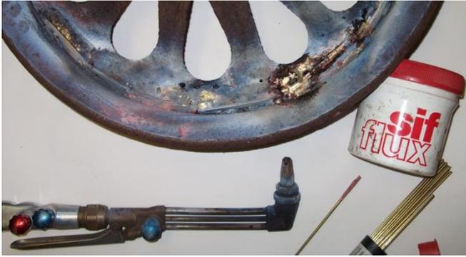
One wheel centre needed patches brazed on near the rim, I am bad at welding thin metal, it disappears, and I find brazing with the oxy-propane much safer.
