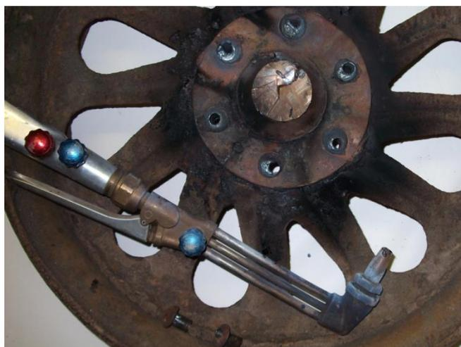
The wheels were cut off with a cutting disc in a 9" angle grinder from the 50mm thick axle, the rivet heads ground off, drilled through and heated with an oxy-propane torch, to break the rust hold. The remains punched out and the boss prised apart, the holes were cleaned with a wire brush and file, then welded up. The welds were then ground back to the original metal thickness.
