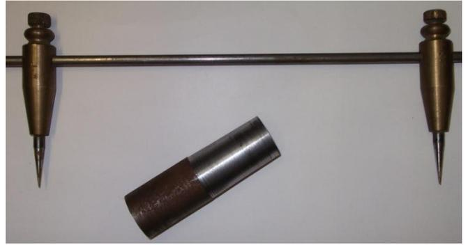
With the taper blank very firmly in the boss you can use a trammel from the centre hole to the rim to re-centre the boss, tack weld it in place, test true running on the actual axle and then re-drill the rivet holes.
