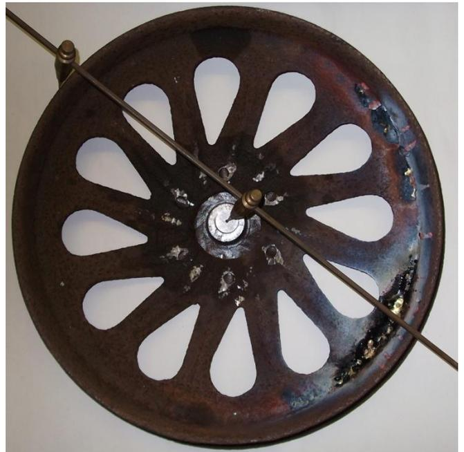
I made 12 rivets to match the holes and re-riveted the two bosses in place. I left the tack welds.
