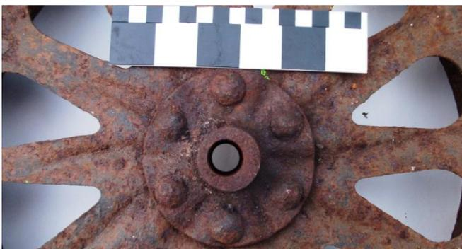
Photos shows two bores off centre, hence the belief the boring was done after the boss was riveted in. Reversing the process involves making a taper blank, to match the bore, and giving this taper blank a centre hole at the small end.
