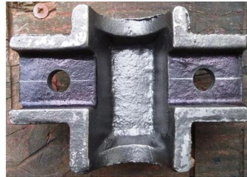
**This is the oil cellar under the half axle bearing, that has the sprung pad in it.**
