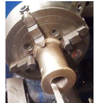
**Two Half bearings being machined, before being split.**
